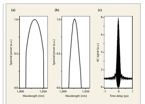
Figure 1. (a) Power spectrum of similariton pulse from numerical simulation. The unusual spectral shape is a signature of self-similar pulse-shaping. (b) Experimental power spectrum produced by Yb fiber laser. (c) Experimental autocorrelation of the dechirped pulse, with duration ~100 fs.
