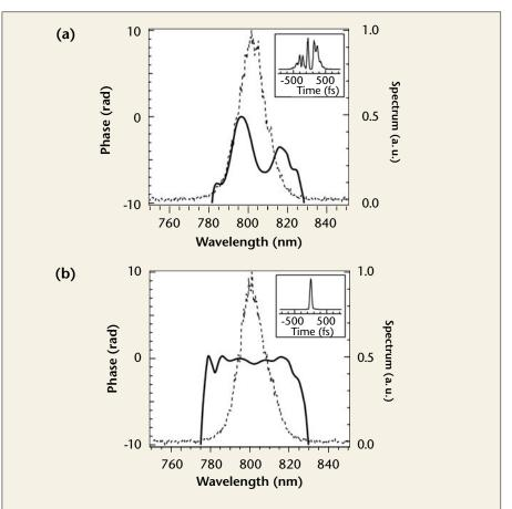
Figure 1. Spectral phase (solid line) and spectrum (dashed line) of our laser pulse passing through cellophane (a) before correction and (b) after correction. The inset shows the corresponding temporal intensity.
